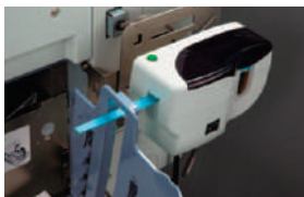
The RISO Job Separator IV:NIII When combined with the "Programmed printing" function, it distinguishes between different printing jobs and separates the printed paper into groups accordingly.
